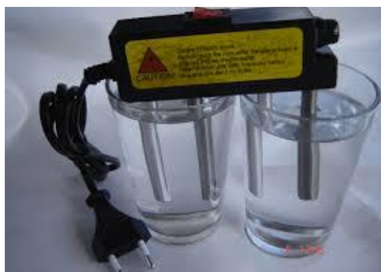
Figure 1. The electrolysis apparatus used by the door-to-door salesman. Note that it can simultaneously electrolyze two solutions. 4
